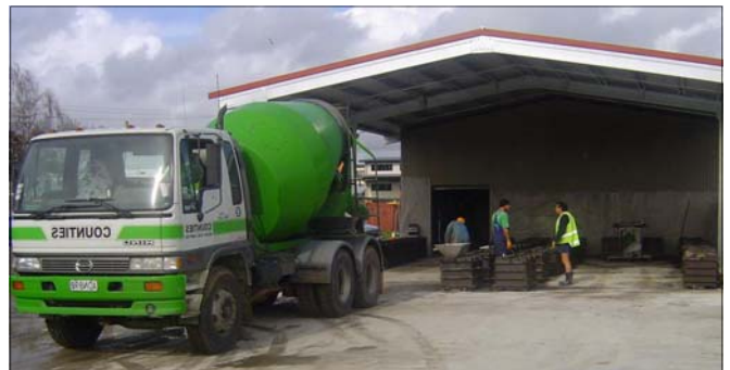
Interlocking block production using residual concrete
