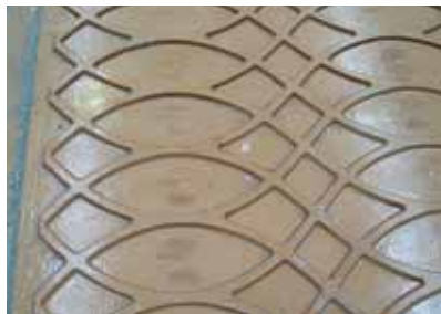
MDF form for precast units.
